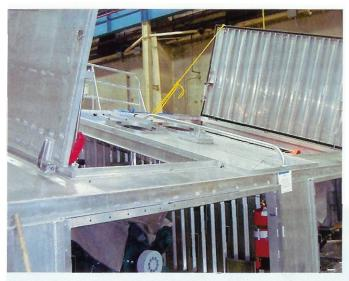
West Coast Insulation and Mascoat use ordinary white vinegar to prep the new aluminum (above). Vinegar is readily available, inexpensive, environmentally friendly, and its slight acidity cleans while removing welding residue. With proper prep, Delta T Marine adheres readily to mullions (window frames, inset, opposite page), which, if left uncoated, would create constant condensation problems.
